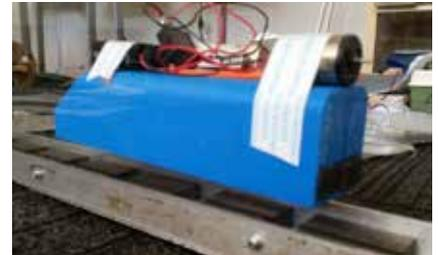
Figure 4: 3D printed propelled prototype train model
